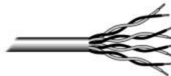
Fig.3. Unshielded twisted pair
